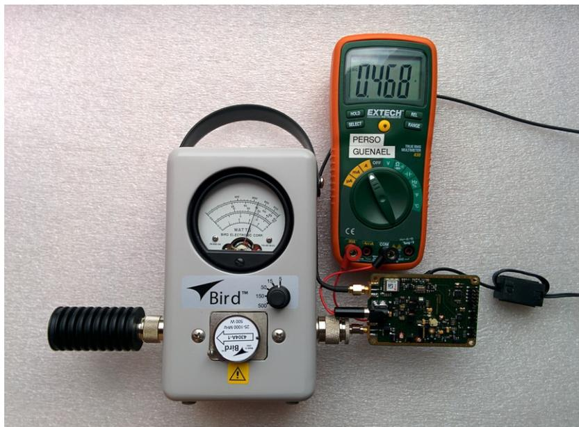
Figure 17: Tuning the circuit by adjusting 2 caps and 1 trimmer
