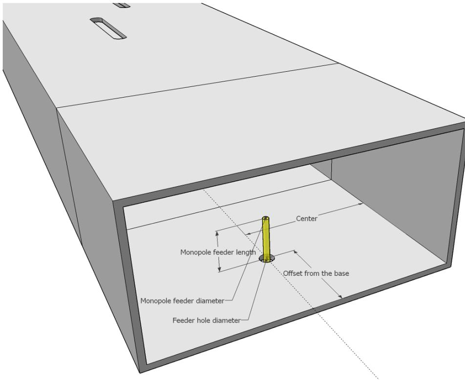
Figure 4: Feeder system
