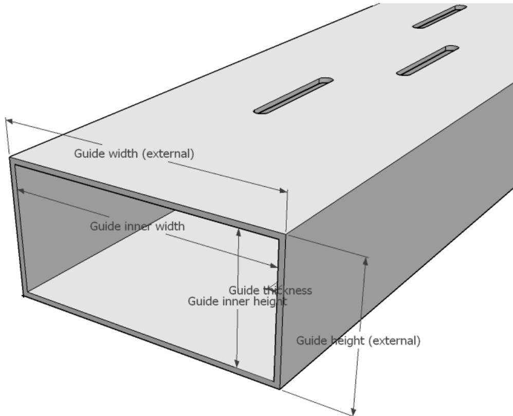
Figure 2: Physical dimensions of the guide
