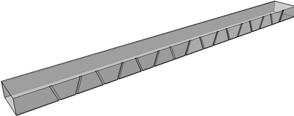
Figure 6: Slot antenna with tilde slots
